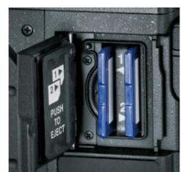
Note: Eye-Fi and FLU cards with wireless LAN functions can be used in SD2 slot.
