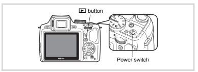
Press the power switch while holding down the button.
