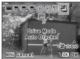
**3** Use the four-way controller ( $\blacktriangle\blacktriangledown$ ) to select EV compensation value and press the OK button.
