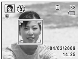
If the camera recognizes a person's face in mode, an orange frame appears showing the area the camera will zoom in to.
