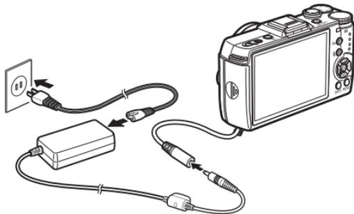
**5 Connect the AC adapter to the AC plug cord, and plug the cord into the power outlet.****Caution**
