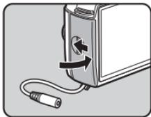
**4 Connect the DC coupler and the AC adapter.**
