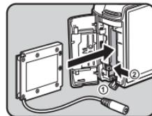
To remove the DC coupler, push the battery lock lever in the direction of ②.
