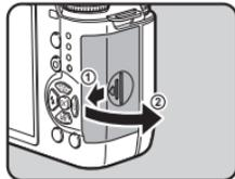
**3 Insert the card all the way with the memory card label facing toward the monitor.**
