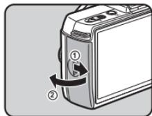
**2** Insert the battery until it locks into place with the ▲ mark facing toward the lens.
