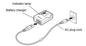
Face the A mark on the battery up, and insert it into the battery charger.
