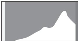
When the image is too dark, the part to the left is cut off (dark portions) and when the image is too bright, the part to the right is cut off (bright portions).
