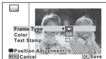
**7** Use the four-way controller (▲▼) to select a frame type, and press the four-way controller (◀).
