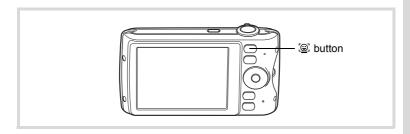
An icon indicating either Face Priority On or Smile Capture appears on the display. (The icon does not appear when the Face Recognition function is not activated.)
