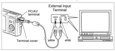
Open the terminal cover and connect the AV cable to the PC/AV terminal.
