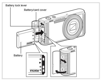
Make sure that the camera is turned off and open the battery/card cover.
