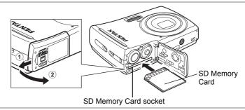
This camera uses either an SD Memory Card or an SDHC Memory Card. (Both cards are referred to as SD Memory Cards hereafter.) Captured images and sound files are saved on the SD Memory Card if a card is inserted in the camera. They are saved in the built-in memory if a card is not inserted.
