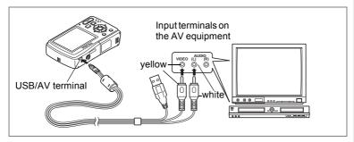
By connecting your camera to a TV or other AV equipment using the supplied USB/AV cable, you can display images on the monitor for review or picture taking.
