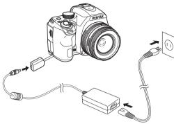
Connect the AC adapter to the AC plug cord, and plug the cord into the power outlet.
