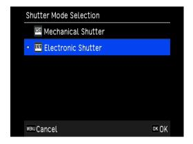
• When electronic shutter is selected, as an additional function shutter speed linkage range is 1/16000 sec. to 30 sec.
