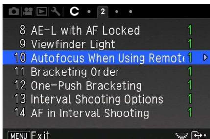
Select [Autofocus When Using Remote Control] in the **C** 2 menu.
