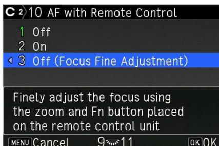
Select [Off (Focus Fine Adjustment)] in [AF with Remote Control].
