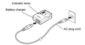
Face the A mark on the battery up, and insert it into the battery charger.
