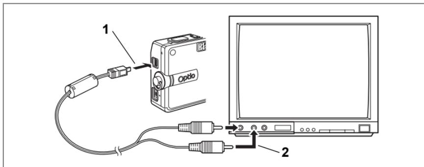
By using the AV cable, you can capture and play back images on a TV or other equipment with a video IN jack. Make sure that both the TV and the camera are turned off before connecting the cable.
