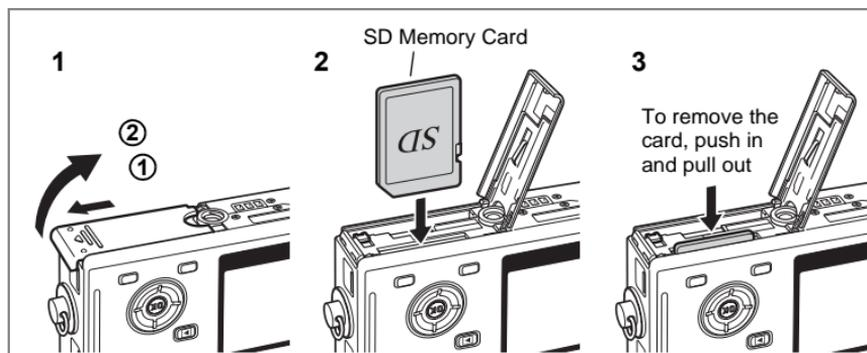
An SD Memory Card can be used with this camera. Captured images are recorded on the SD Memory Card if a card is inserted or in the built-in memory if no card is inserted.
