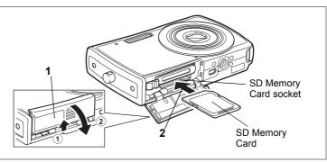
This camera uses an SD Memory Card. Captured images and sound files are saved on the SD Memory Card if a card is inserted in the camera. They are saved in the built-in memory if a card is not inserted. (p.32)
