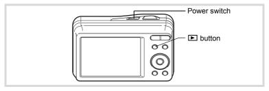
Press the power switch while holding down the **\bigsilon** button.
