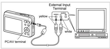
Connect the AV cable to the PC/AV terminal.
