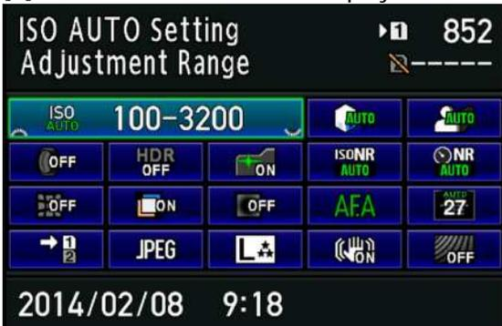
[3] Move the selection frame (green) that is overlaid on [ISO AUTO Setting] in the illustration above using the four-way controller (↑ ↓ ← →) to [Anti-Aliasing Filter Simulator] in the lower right corner of the screen.
