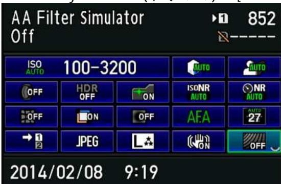
[4] The Anti-Aliasing Filter Simulator setting switches in the following order by turning the rear e-dial counterclockwise: [OFF] → [TYPE1] → [TYPE2] → [Bracketing] → [OFF].
