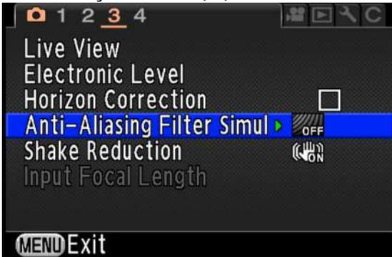
[3] As shown below, a pop-up menu with a green frame appears if the four-way controller (→) is pressed when the selection frame is placed over [Anti-Aliasing Filter Simulator].
