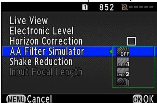
[4] The pop-up menu shows four options in the following order: [OFF], [TYPE1], [TYPE2] and [Bracketing]. Use the four-way controller (↑) or (↓) to select [Bracketing] and press the OK button.
