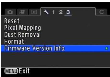
[6] Press the four-way controller right to display [Firmware Version Info].
