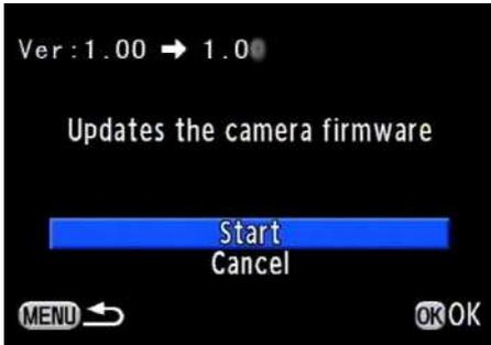
\*If firmware file is not saved to SD/SDHC card correctly, this screen will not be displayed.
