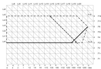
• When [Program] is selected in [One Press M Mode] of the [Key Custom Options] menu (P.42), the aperture value and shutter speed are adjusted according to the [P Mode Selection] setting you set.
