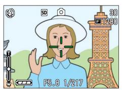
Once the shot is in focus, the exposure and white balance are fixed and the crosshair in the center of the LCD Monitor turns green, as does the auto-focus lamp in the lower left of the Viewfinder. Check one of these to make sure the subject is in focus.
