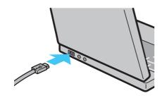
Open the terminal cover, and then connect the USB cable to its USB terminal.
