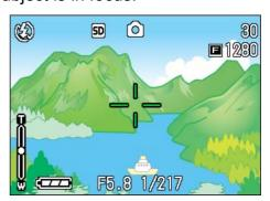
If the camera cannot automatically focus, the crosshairs in the center of the LCD monitor turn red and the auto-focus lamp in the lower left of the viewfinder blinks in green.
