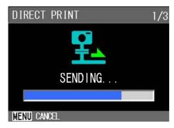
Press the MENU button to cancel. At the end of transmission, the display returns to the Direct Print playback mode screen and printing starts.
