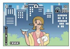
The flash starts recharging. While the flash is charging, the LCD Monitor goes off and the flash lamp blinks. Once charging is complete, the lamp goes off and it is possible to shoot.
