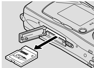
The card eject function is activated by pushing the card in. Keep the card horizontal when pulling it out.
