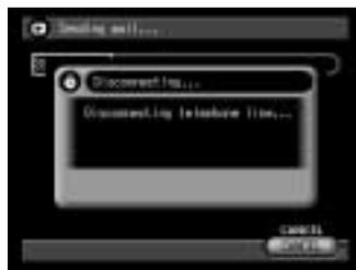
When uploading is finished, the connection will be automatically terminated and the screen will return to the Edit mode.
