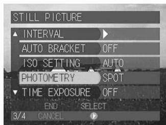
3 Choose the exposure metering system (CTR WGHT, SPOT or MULTI) and then press the ENTER button.
