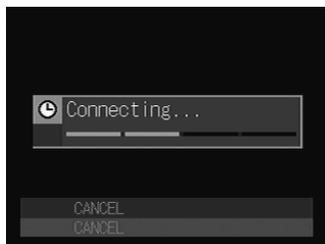
The mark at the top of the LCD panel will rotate clockwise while the connection is established.
