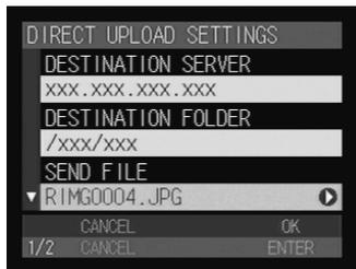
The image that has been selected to be uploaded is marked with a green
