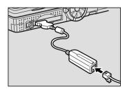
6 Insert the end of the modular cable into the modular jack.
