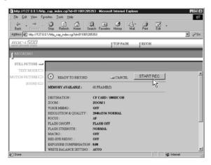
Shooting is performed after approximately 10 seconds and the image is displayed in a reduced state with information such as the shooting date, etc. (A short time is required to transmit the image.)
