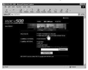
After a short while, the data recorded in the internal memory will be displayed in thumbnail form (it may take a while for the data to be transmitted from the camera).
