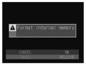
Press the shutter release button again. The "Formatting ..." message will be displayed, and when formatting is completed, the display will return to the Setup menu.
