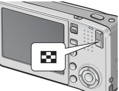
The screen changes to three-frame view. The large frame at the center of the screen displays the currently selected still image.
