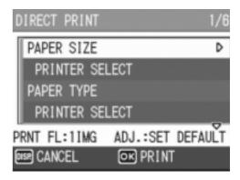
The following items can be selected. Each item appears only when supported by the printer connected to the camera.
