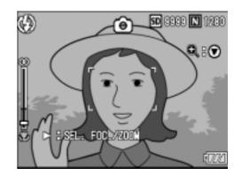
3. Press the [4] (Telephoto) button or the [4] (Wide-angle) button to adjust the focus.
