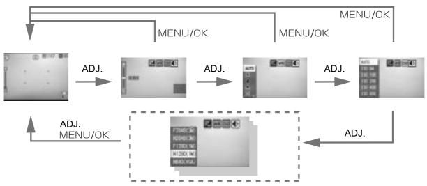
Use the SETUP menu to assign a function to the ADJ. button (P.115).
