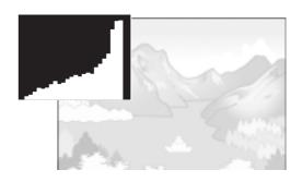
If the histogram has only peaks on the left side without anything else, this picture is under-exposed with too many pixels only for shadow sections.
