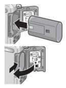
Removing the Rechargeable Battery.
