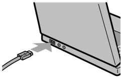
3. Connect the USB cable to the USB terminal of your camera. Your camera turns on.
