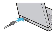
3. Connect the cable to the camera USB terminal.
