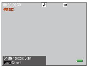
Recording ends after 30 seconds or when the shutter-release button is pressed halfway. The description list will be displayed with a ▶ icon next to the [Record] option (in playback mode, [Record] changes to [Playback]).
