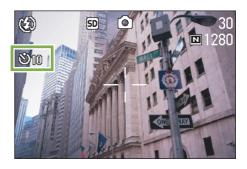
3 Press the shutter release button. The flash begins to blink and the Self-timer starts. After about ten seconds the camera takes the picture. About two seconds before it shoots, the time interval between blinks begins to shorten and the audio tone begins to beep.
