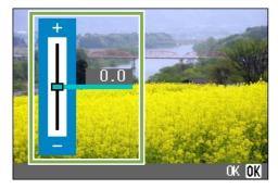
4 Press the ▲▼ buttons and specify a value. Moving it to the - (minus) side makes darker. Moving it to the + (plus) side makes it brighter.
