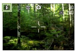
The flash starts recharging. While the flash is charging, the LCD Monitor goes off and the flash lamp blinks. Once charging is complete, the lamp remains lit and it is possible to shoot.
