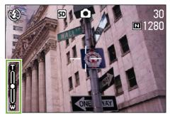
With the subject image enlarged to the end of the T side (Telephoto) on the Zoom Bar, release the 1 button once and press 1 button again and hold down.
