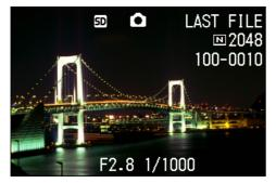
Press the (Thumbnail Display) button. The screen is split into six sections. Still images and movies (the first frame) are displayed in a reduced size.
