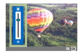
4 Press the ▲▼ buttons to adjust the brightness.
