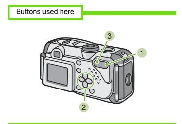
Press the Q (Enlarged View) button. The still image is enlarged. One part of the still image is displayed on the LCD Monitor. The enlargement ratio changes each time you press
