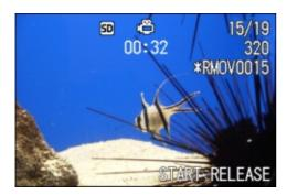
3 Press the shutter release button. Playback begins. The elapsed playback indicator or the elapsed time is displayed on the LCD Monitor.
