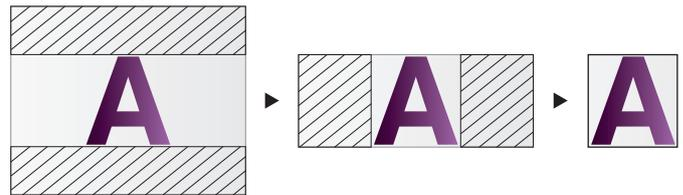
Transfer time reduced by sending only areas necessary for inspection
